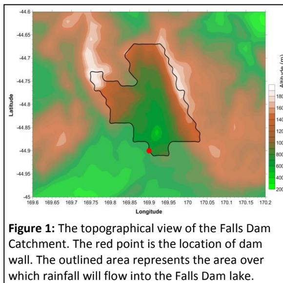
**Figure 1:** The topographical view of the Falls Dam Catchment. The red point is the location of dam wall. The outlined area represents the area over which rainfall will flow into the Falls Dam lake.
